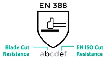
The EN388 shield pictogram can report up to 6 separate mechanical performance measures. The original Blade Cut test score in position “b” is measured on a scale of 0-to-5 as determined by the EN Coup test. The new EN ISO Cut Resistance score in position “e” measures on a scale of A-thru-F.
